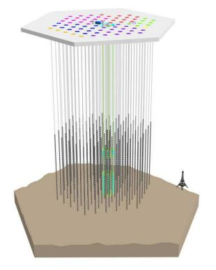
Figure 1: A schematic view of the IceCube detector, with the Eiffel Tower also shown for scale. The colors of the dots where each string connects to the surface of the glacier represent the year in which that string was deployed.
