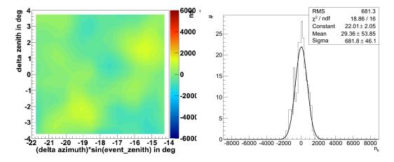
Figure 3: Left: fluctuations around the background model of an off-source region, defined in relation to the position of the Moon. The color axis is the best-fit number of total signal events given the response at that point. Right: the distribution of bins from the left plot, which can be fit to a gaussian curve, confirming that the background is fluctuating randomly around 0. From [3].
