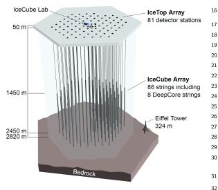
**Fig. 1**: The IceCube neutrino detector in the Antarctic ice. $^{33}_{34}$  A picture of the Eiffel Tower is shown for scale.  $^{35}$
