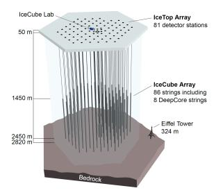
**Fig. 1**: The IceCube neutrino detector in the Antarctic ice. A picture of the Eiffel Tower is shown for scale.
